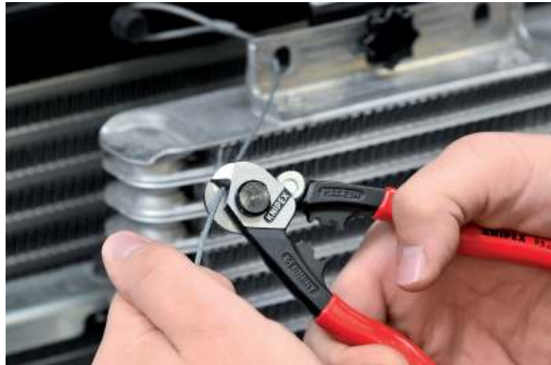
Crimping of the end caps on the Bowden cable sheath
