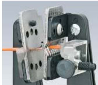
Automatic stripping of the insulation
