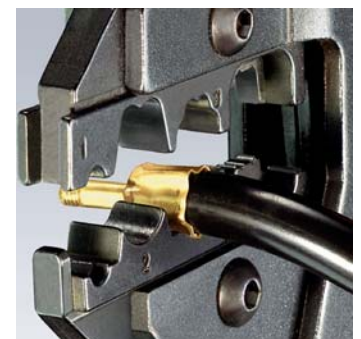
43 200 with crimping dies 97 49 35 for spark plug connectors
