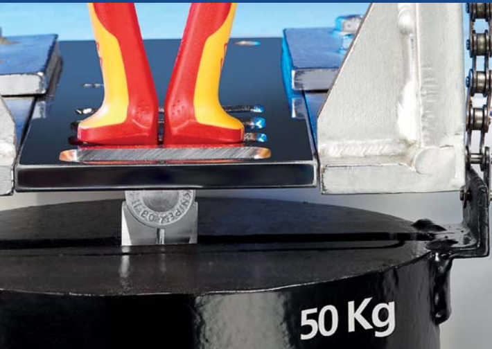
Testing the adhesion of the insulating coating at 500 N.
