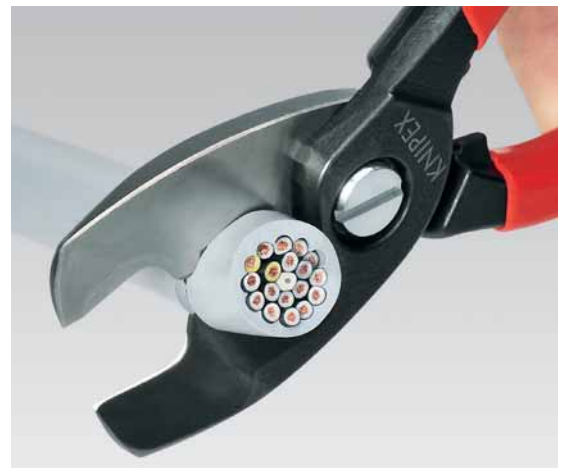
Final cut: after cutting the sheath in the front profile the conductors in the rear part are cut. Initial cut in the front profile, final cut in the rear profile – to keep it as easy as possible.
