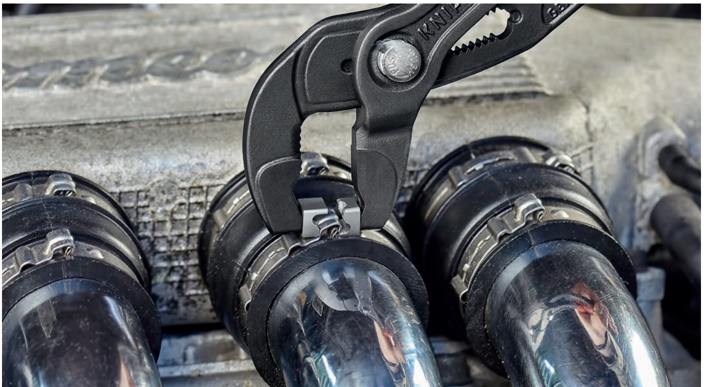
Opening a hose clamp without limit stop
