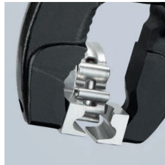
Opening a hose clamp with limit stop
