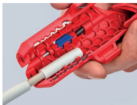
Dismantling of a NYM cable
