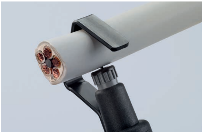
Setting the tool for circular cut
